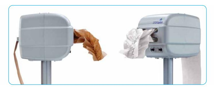
Three operating modes also simplify on-demand production of paper cushioning directly at the packing station, while the system itself features a compact, space-saving design. A silo and a single PAPERplus® Papillon can supply multiple packing stations with cushioning at the same time. The paper used by PAPERplus® Papillon to create paper cushioning is available in brown and several other colors.
